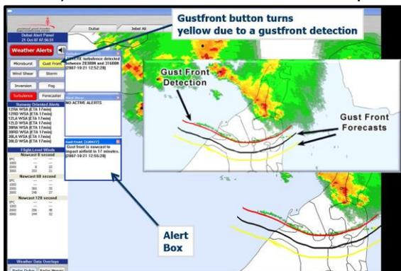
**Figure 2.** Example of AWDSS display in Dubai showing output from the gust front detection algorithm and automated altering (left panels).
