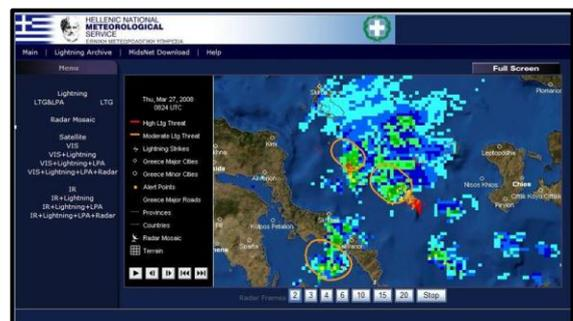
**Figure 4.** Example of HNMS LDSS display showing lightning activity, predictions, and radar data.
